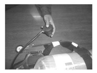
Check whistle setting by closing the cylinder valve and opening bypass very slightly to vent air from the system. Slowly check that the whistle sounds clearly at the correct pressure. If necessary reset whistle.
