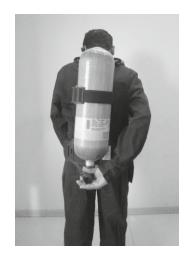
**1.3** Check that demand valve is switched off (depress reset button) and turn on cylinder valve slowly. Check cylinder contents by reading pressure guage.
