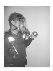
**3.3** If no leak is detected open cylinder valve fully and check operation of bypass for a good flow of air.
